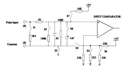
The Frequency Input Circuit
